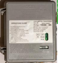
A green light on the LCT means the device is working and is not currently controlling your water heater or other device.
